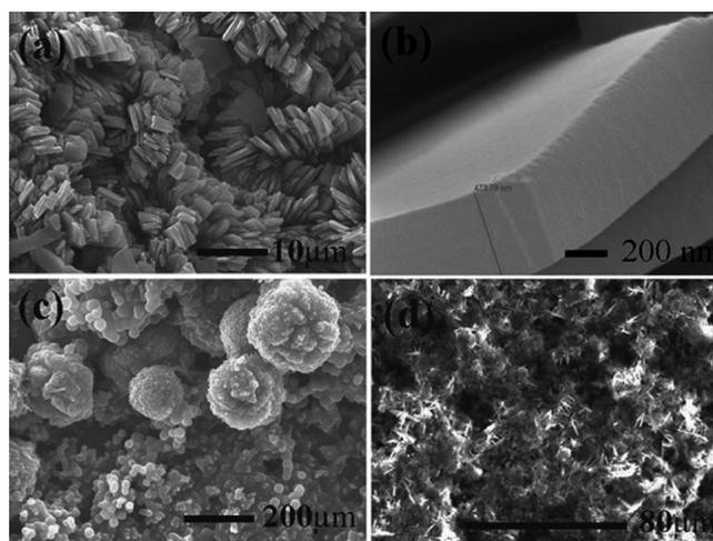
**Figure 4.** SEM images of Pd nanoparticles. Reprinted with permission from ref 65. Copyright 2009 the Royal Society of Chemistry.
