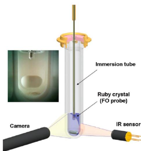
**Figure 2.** Schematic view of the utilized microwave cavity highlighting dual external (IR) and internal (FO) temperature control and the location of the built-in camera. The inset shows an image taken by the camera (2 mL liquid volume, magnetic stir bar).<sup>33</sup> Reprinted with permission from ref 33. Copyright 2013 WILEY-VCH Verlag GmbH & Co. KGaA.
