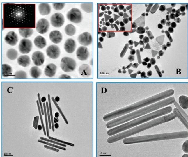
**Figure 11.** TEM image of different shaped Au NPs after 90 s of MW exposure: (A) image of spherical Au NPs; (B) low magnification images of mixed shaped gold NPs; (C, D) images of Au nanorods at different magnification. The insets of panels A and B show the corresponding electron diffraction of the particles and a higher magnified image. Reprinted with permission from ref 73. Copyright 2008 American Chemical Society.
