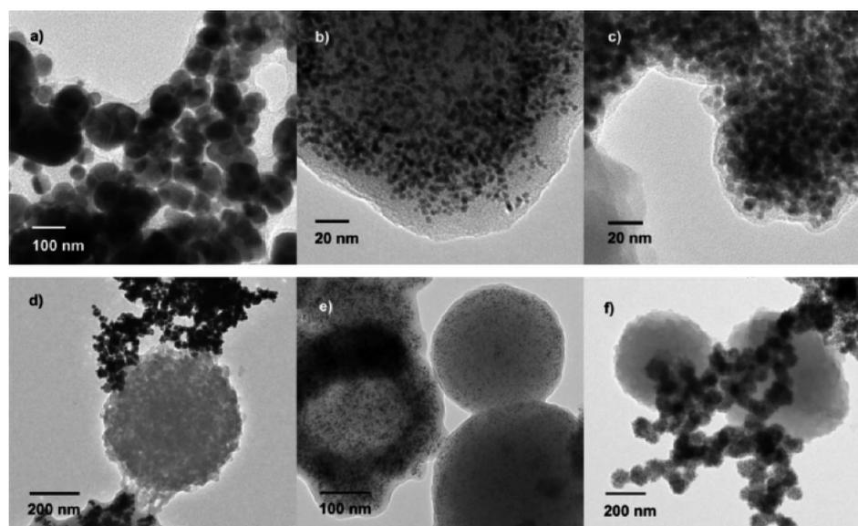
**Figure 9.** TEM images of typical Au, Pt, and Pd samples: (a) Au with capping; (b) Pt with capping; (c) Pd with capping; (d) Au with organic microspheres; (e) Pt with organic microspheres; (f) Pd with organic microspheres. Reprinted with permission from ref 72. Copyright 2012 the Royal Society of Chemistry.
