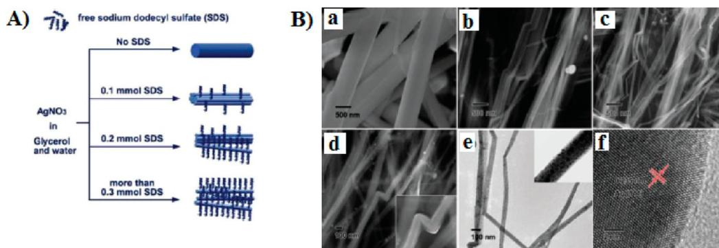
**Figure 6.** (A) Illustration of the formation process of Ag nanowires in the presence of SDS. (B) (a–d) SEM images of the Ag samples with different SDS amount (other chemicals, 0.3 mmol  $\text{AgNO}_3$ , 4 mL of glycerol, and 4 mL of water): (a) no SDS; (b) 0.1 mmol SDS; (c) 0.2 mmol SDS; (d) 0.3 mmol SDS. (e) TEM and (f) HRTEM images of typical Ag nanowires. Reprinted with permission from ref 69. Copyright 2013 the Royal Society of Chemistry.
