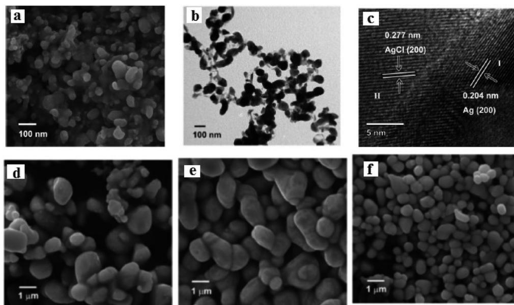
**Figure 8.** Images of AgCl/Ag NPs prepared with beet juice: (a) SEM image, (b) TEM image, and (c) HRTEM image. SEM images of (d) sample obtained after MW irradiation with glucose, (e) sample obtained after MW irradiation without any reducing reagent, and (e) AgCl obtained before MW irradiation. Reprinted with permission from ref 71. Copyright 2012 WILEY-VCH Verlag GmbH & Co. KGaA.
