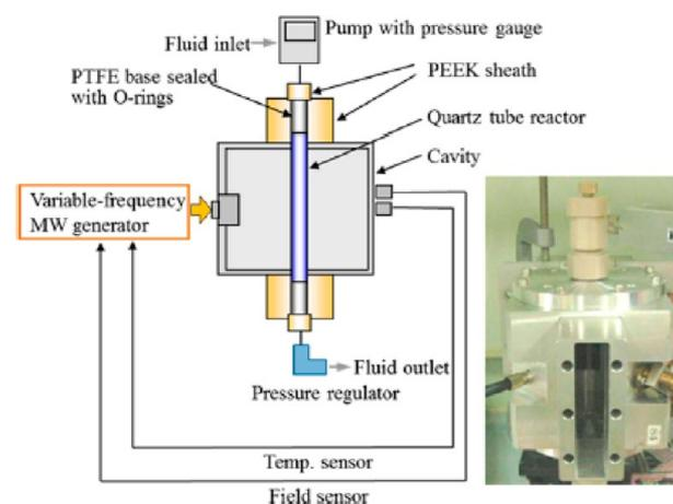
**Figure 3.** Experimental setup of the present MW-assisted flow reactor system and a photograph of the MW cavity part. The quartz reactor tube is connected with the PEEK sheath, which is designed to resist up to 10 MPa. Reprinted with permission from ref 26. Copyright 2013 American Chemical Society.
